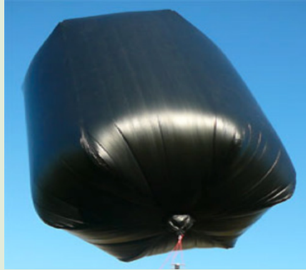
Fig 4.8: A simple solar balloon.
